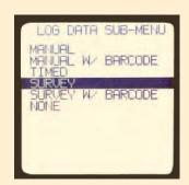
Programming of survey sequences, as well as retrieval of logged data, is accomplished via the built-in IrDA port.
