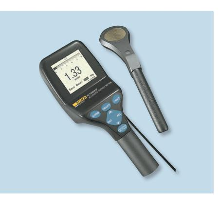
The ASM–990 Series Advanced Survey Meter can detect alpha, beta, gamma, or x-ray radiation within an operating range of 1  $\mu$ R/hr to 1 R/hr (1 to 5,000,000 CPM), depending on the selected probe (Geiger–Mueller, neutron, proportional counter, scintillation). With the proper probe combination, this meter can be used as a general survey meter, an area monitor, a wipe–test counter, and a contamination monitor.
